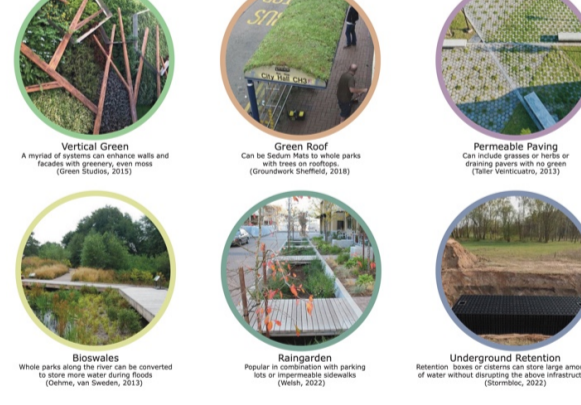
Vertical Green A myriad of systems can enhance walls and facades with greenery, even moss (Green Studios, 2015) Green Roof Can be Secum Mats to whole parks with trees on rooftops (Groundwork Sheffield, 2018) Permeable Paving Can include grasses or herbs or planting plants with no grass (Taller Venturolo, 2013) Bioswales Whole parks along the river can be converted to store more water during floods (Dierke, van Steenbeek, 2013) Rain garden Popular in combination with parking lots or impermeable sidewalks (Wolke, 2012) Underground Retention Basins or cisterns can store large amounts of water without disrupting the above infrastructure (Gronwald, 2022)
