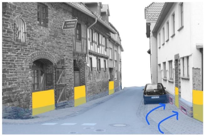
Waterproof doors and Floodable basements
