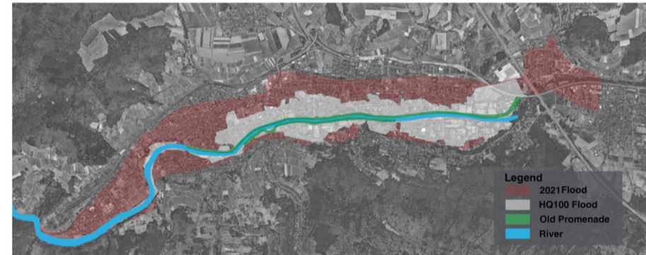
Designing the new promenade according to the HQ100 flood line and 2021 flood
