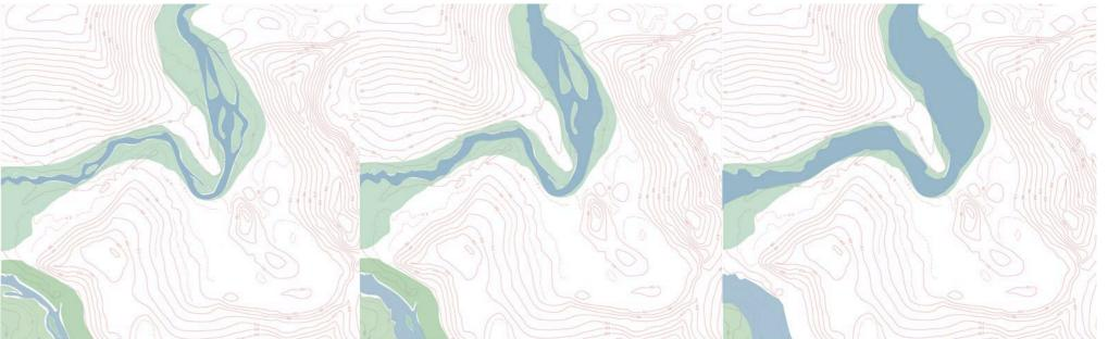
When making the riverbed wider, it slows down the water and can under hevy water flow store a larger amount. This is important to do in the areas where it is room for this possibility.
