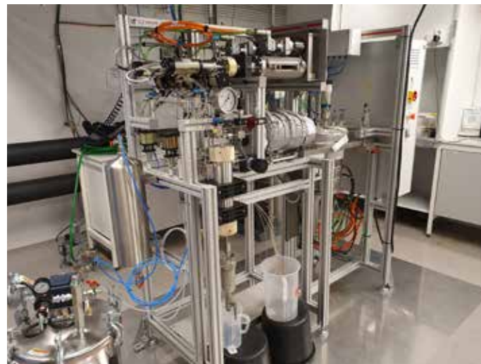
SINTEF Energy's lab-scale HTL mini-pilot system
