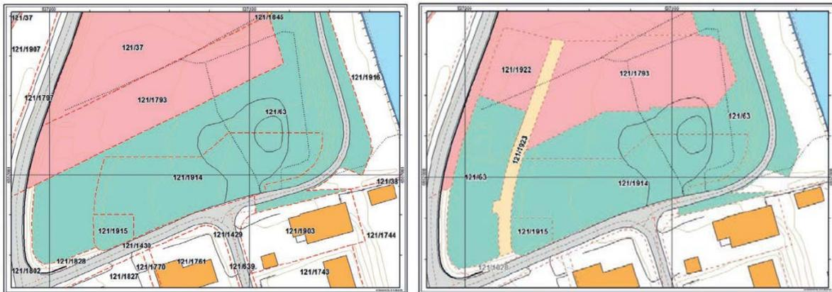
**Figure 1:** Part of a land consolidation map in an urban area. Before land consolidation (left) and after land consolidation (right) in the municipality of Porsgrunn (Nedre Telemark Land Consolidation Court, case: JSKI-2007-68).
