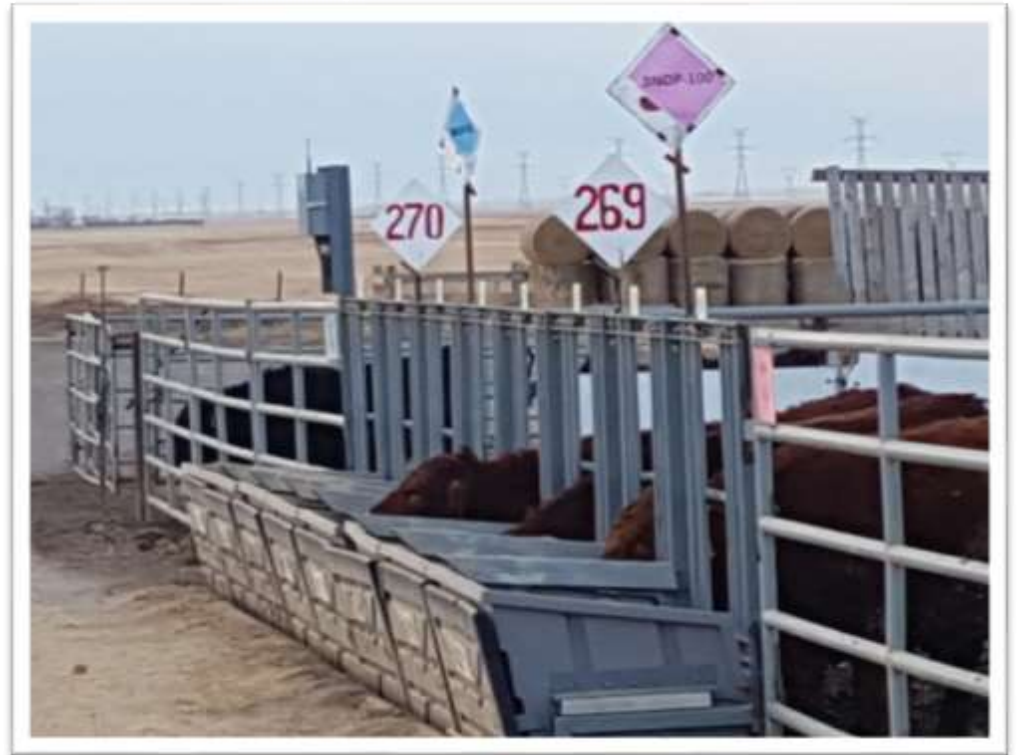
GrowSafe system to measure feed intake per animal
