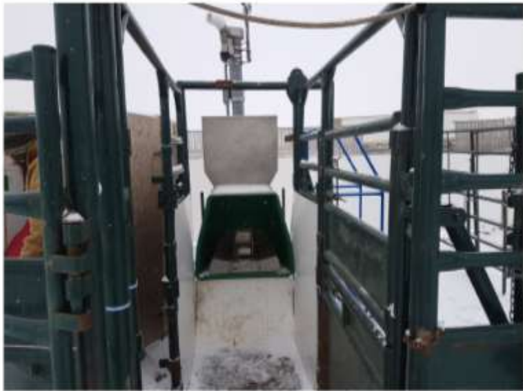
GreenFeed System to measure methane production per animal
