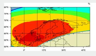
**Figure 7:** Map with probability of arrival of radioactive cloud to a given location from a hypothetical accident in the Sellafield nuclear facilities.
