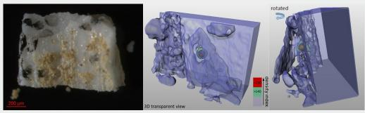
**Figure 4:** Retention of a U/Pu particle in snails at Palomares. A) Piece of snail shell contaminated with <sup>241</sup>Am. B) Nano-CT rendering of the shell piece showing the 10 μm U/Pu particle as high absorption material (reddish brown). C) The tomographic rendering in C rotated to show the particle partially embedded within the shell.
