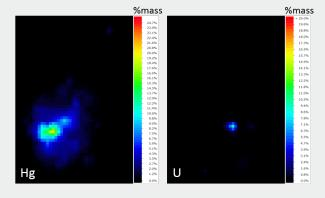
*Figure 5:* Micro-XRF (M4 Tornado, Bruker Nano) quantitative mapping of Hg and U in a heterogeneous particle isolated from Ottawa River sediments originating from the Chalk River nuclear site. Elements identified include: Cr, Ni, Cu, Zn, As, Zr, Hf, Mo, Hg, Pb and Th as well as U. Bar 1 mm.
