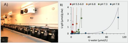
*Figure 10: A)* Design juvenile exposure, *B)* Relationship between *U* in unfiltered water and accumulation in gills
